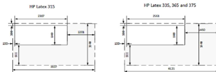
The space required for the cutter is illustrated below (measurements in millimeters):
