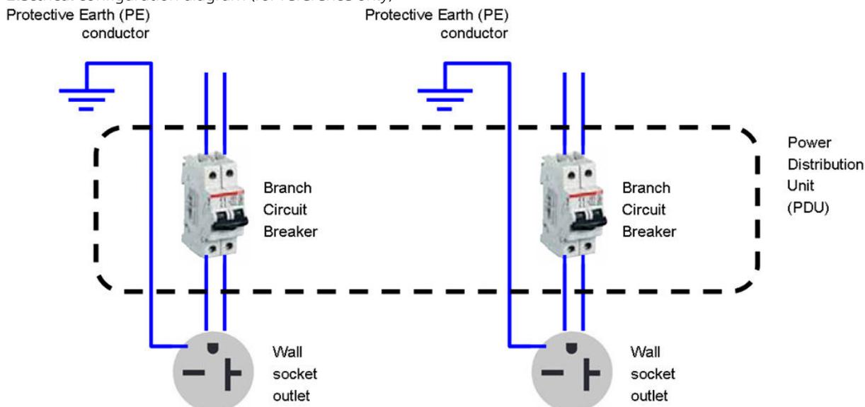
**NOTE:** The Power Distribution Unit (PDU) must be rated to meet the power requirements of the printer, and shall be in accordance with the Electrical Code requirements of the local jurisdiction of the country where the equipment is installed.
